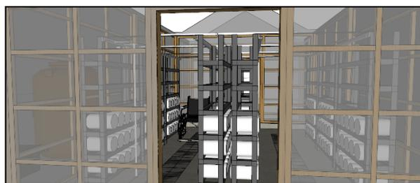
Fig. 4. The earliest structure proposal of the misting system for one level mushroom baglogs
