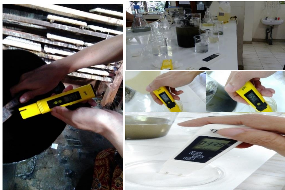
Fig 6. pH and TDS testing for filtered water in laboratory environment
