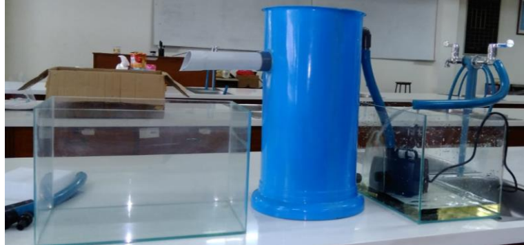
Figure 7. Filtration system that is used in tofu production system
