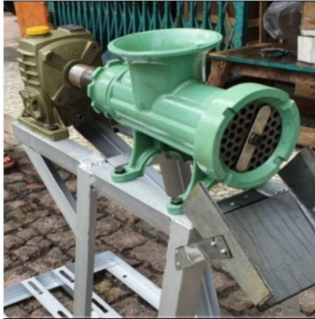
Fig. 5. Milling tools for fish feed ingredients Milling is done when the material is still in a soft position so that it is easy to process and grind it into fish feed ingredients
