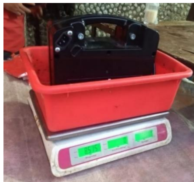
Figure 10. Electric wheelchair type B battery weight measurement
