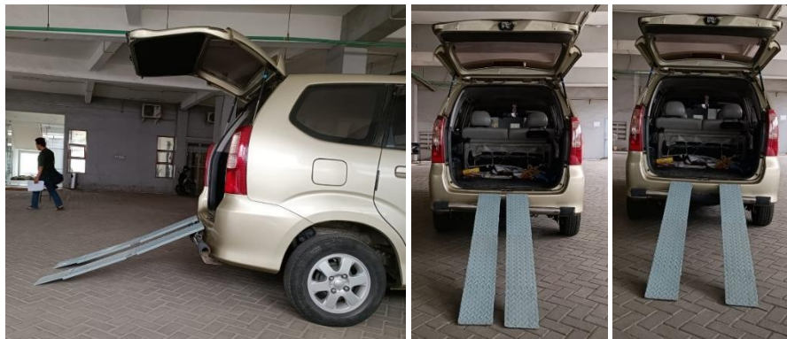
Figure 17. Installation of inclined plane base on the car
