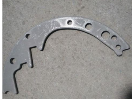
Gambar 3. Elemen brake shoe : stang
