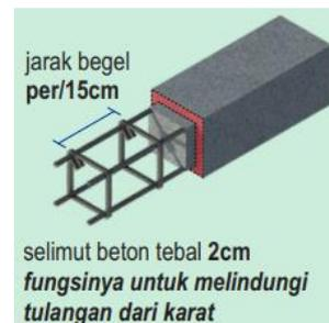
**Gambar 21.** Jarak Sengkang Balok
