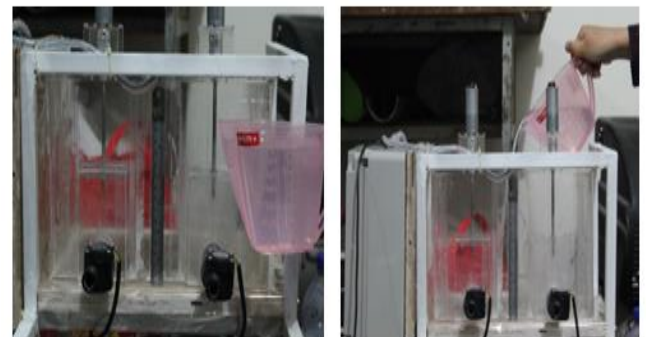
Gambar 29. Pengujian water flow sensor
