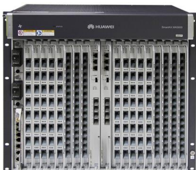
Gambar 4 OLT ( Optical Line Terminal )
