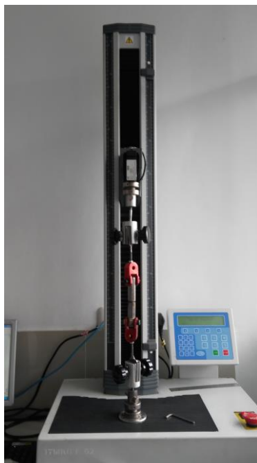
Figure 2. Samples are ready for tensile testing on Instron machines.
