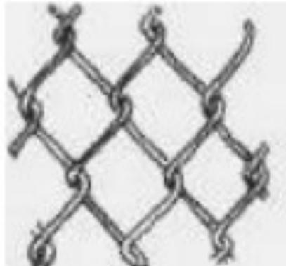
Gambar 7 Vertikal single hook braiding
